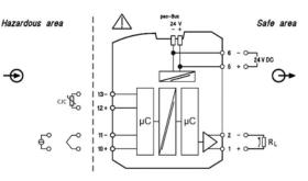
The Temperature Transmitter is an associated apparatus as well as a nonincendive apparatus for installation in SAFE AREA and provides intrinsically safe circuits for field devices located in HAZARDOUS AREAS.
