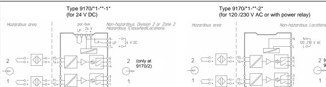
The Switching Repeater Type 9170/\*1-\*d-1\* (d = 0, 1, 4) is an associated apparatus as well as a nonincendive apparatus for installation in non-hazardous or Class 1, Division 2 or Zone 2 Hazardous (Classified) Locations and provides intrinsically safe connections for one (or two) field devices located in Class I, II, III, Division 1, Group A-G or Class I, Zone 0 [AEx ia] Group IIC, hazardous locations according to NEC Article 504/505 as listed below.
