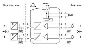
The Isolating Repeater Output is an associated apparatus as well as a nonincendive apparatus for installation in SAFE AREA and provides intrinsically safe circuits for field devices located in HAZARDOUS AREAS.
