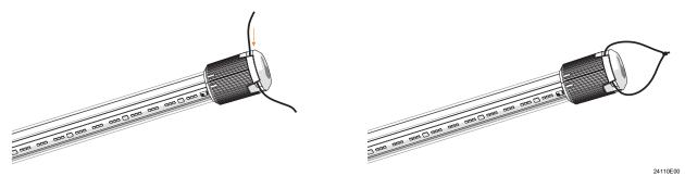
▶ Use the ex-factory anti-fall mechanism.
