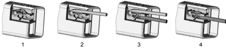
Figure 8-1: Cable connection to screwless terminals
