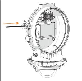
Insert the conductor and connect it to the luminaire (electrical connections, see chapter 7.3.2; cable entries, see chapter 7.3.3)
