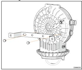
Screw the mounting bracket into the intended threaded holes.
