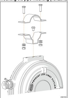
Screw the pipe clamp into the intended threaded holes.
