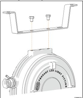
Screw the mounting bracket into the intended threaded holes.
