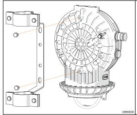
Screw the pipe clamp into the intended threaded holes.
