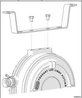
Screw the mounting bracket into the intended threaded holes. The mounting bracket can be used to suspend the luminaire from the ceiling.
