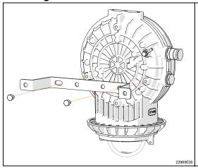
Screw the mounting bracket into the intended threaded holes. The mounting bracket can be used to fasten the luminaire on walls.
