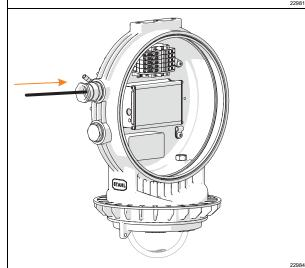
Insert the conductor and connect it to the luminaire (electrical connections, see chapter 7.3.2; cable entries, see chapter 7.3.3)
