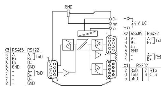
The Fieldbus Isolating Repeater Type 9185/11-\*\*-10 is an associated apparatus as well as a nonincendive apparatus for installation in Non-Hazardous, Class I, Division 2 or Zone 2 Hazardous (Classified) Locations providing intrinsically safe connections for one field device located in Class I, II, III, Division 1, Group A-G or Class I, Zone 1 [AEx ib] Group IIC, Hazardous Locations according to NEC Article 504/505 as listed below.
