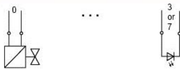
Approved intrinsically safe solenoid valves, indicating lamps
