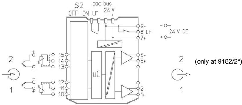
The Temperature Transmitter Type 9182/\*0-5\*-6\* is a nonincendive apparatus located in a non-hazardous or Class 1, Division 2 or Zone 2 Hazardous (Classified) Location.
