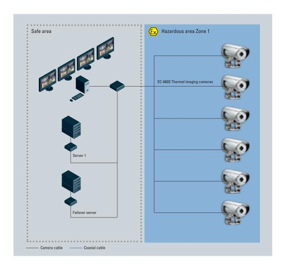
This CCTV project involved monitoring the surface of four large tanks with four thermal imaging cameras each. Previously, this had been done by means of actual inspection rounds.
