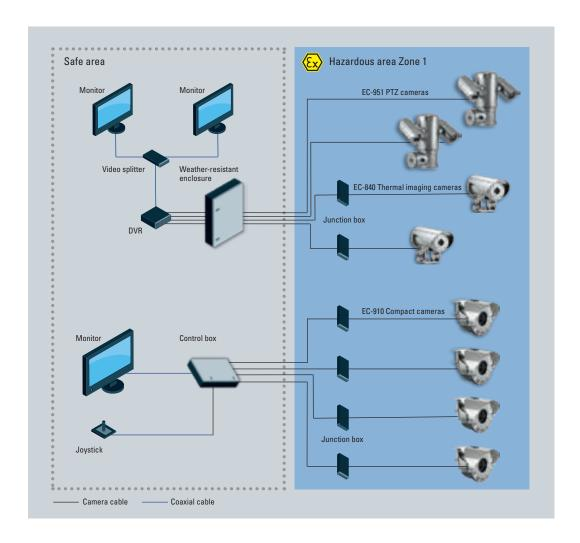
This project for an offshore rig involved a combined surveillance solution for the drill pipe, certain gas and fire detectors and other critical areas on the rig.
