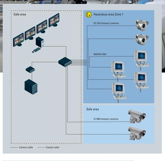
For this pharmaceutical production plant, the light-sensitive EC-910 compact camera attached to sight glass mounts constitutes the central means of monitoring the production tanks.
