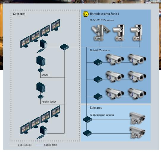
The large volume of highly flammable hazardous substances present in the production areas of a refinery make explosion-protected cameras in addition to cameras in safe areas an absolute necessity.
