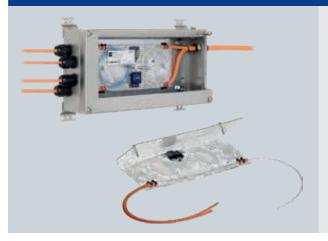
The 8186 FO splice cassette with type of protection "op pr" (see IEC EN 60079-28) is used for the correct and fast connection of 6 or 12 fibre optic cables in hazardous areas.
