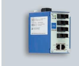
The 9721 switch is used for linking electrical Ethernet networks with optical 100 Mbps Ethernet networks. With type of protection "op is", the 4 FO ports are designed for operation in hazardous areas (see IEC EN 60079-28). This way, conventional fibre optic cables can also be used in hazardous areas and may be connected and disconnected during operation (hot plug).
