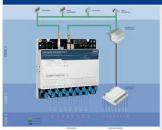
The Ethernet-APL field switches series 9740 are intended for the connection of intrinsically safe 2-WISE field devices to superordinate 4-wire Ethernet networks, and supply the devices with intrinsically safe power. The field switches can be installed in Zone 1 or Zone 2.
