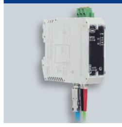
The Ethernet media converters for installation in Zone 1 convert Ethernet via fibre optics (FX) to Ex i Ethernet via CAT cable (TX). With this converter, industrial CAT cables can be plugged and unplugged during operations also in Zone 1 (hot plug). The devices are particularly suitable for operation of the Zone 1 Remote I/O IS1+.
