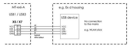
Type 1 connection diagram (e.g. WLAN stick)
