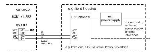
Type 2 connection diagram (e.g. hard disk, CD / DVD with power supply)
