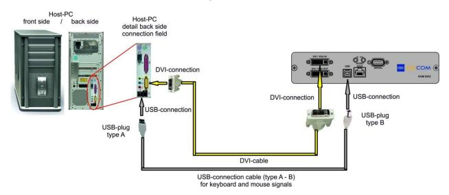
If the host computer has no DVI video signal, the KVM transmission unit can also be connected via a VGA video signal and cable. In this case, however, each host PC resolution used requires a video calibration of the KVM transmission unit.
