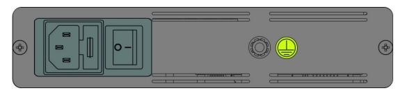
Dimensions in mm / ft:  $210 \times 44.45 \times 165 / 0.689 \times 0.146 \times 0.541$  (W x H x D)
