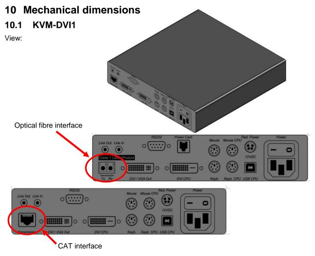
Dimensions in mm / ft:  $210 \times 44 \times 210 / 0.689 \times 0.144 \times 0.689 \text{ (W x H x D)}$
