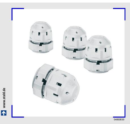
Breathers provide continuous pressure equalisation between the inside of the enclosure and the atmosphere around the enclosure. This prevents moisture from entering the enclosure via the seals and condensing inside the enclosure.
