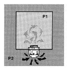
Pressure differences between the inside of the enclosure (P1) and the surrounding atmosphere (P2) due to temperature are reliably equalised by the breather. This minimises the build-up of condensation in the enclosure.
