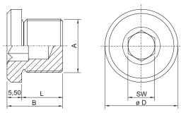
$A = Thread \ size \quad B = Length \quad L = Thread \ length \\ D = Outer \ diameter \quad SW = Width \ across \ flats$
