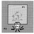
Temperature-related pressure differences between the inside of the enclosure (P1) and the surrounding atmosphere (P2) are balanced by the breather. The amount of condensation forming in the enclosure is thus kept to a minimum.
