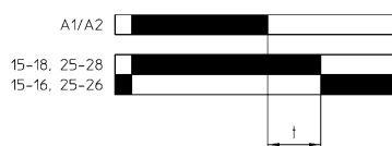
OFF delay relay without power supply Timing range: 0.05 s to 10 min
