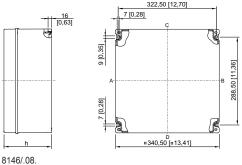
8146/.08. 8146/.081: h = 91 mm [3.58 inch] 8146/.082: h = 131 mm [5.16 inch] 8146/.083: h = 150 mm [5.91 inch] 8146/.084: h = 171 mm [6.73 inch] 8146/.085: h = 190 mm [7.48 inch] 8146/.086: h = 230 mm [9.06 inch]
