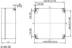
8146/.08. 8146/.081: h = 91 mm [3.58 inch] 8146/.082: h = 131 mm [5.16 inch] 8146/.083: h = 150 mm [5.91 inch] 8146/.084: h = 171 mm [6.73 inch] 8146/.085: h = 190 mm [7.48 inch]
