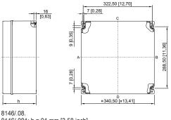
8146/.08. 8146/.081: h = 91 mm [3.58 inch] 8146/.082: h = 131 mm [5.16 inch] 8146/.083: h = 150 mm [5.91 inch] 8146/.084: h = 171 mm [6.73 inch] 8146/.085: h = 190 mm [7.48 inch] 8146/.086: h = 230 mm [9.06 inch]
