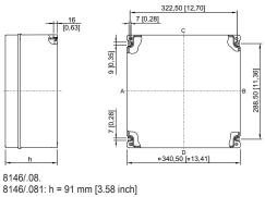
8146/.081: h = 91 mm [3.58 inch] 8146/.082: h = 131 mm [5.16 inch] 8146/.083: h = 150 mm [5.91 inch] 8146/.084: h = 171 mm [6.73 inch] 8146/.085: h = 190 mm [7.48 inch]
