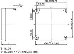
8146/.081: h = 91 mm [3.58 inch] 8146/.082: h = 131 mm [5.16 inch] 8146/.083: h = 150 mm [5.91 inch] 8146/.084: h = 171 mm [6.73 inch] 8146/.085: h = 190 mm [7.48 inch] 8146/.086: h = 230 mm [9.06 inch]
