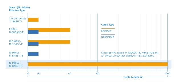
Figure 3: Ethernet-APL and Types of Single-Pair Ethernet defined in IEEE 802.3
