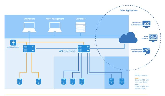
Figure 6: Networking the entire automation pyramid
