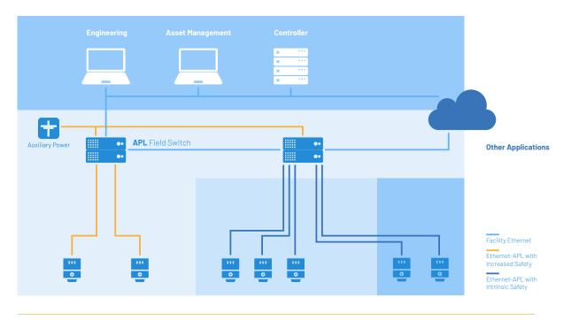
Figure 4: Example topology for a compact star installation
