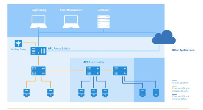
Figure 5: Example topology for long cable reach with up to 1000 m between switches on the trunk
