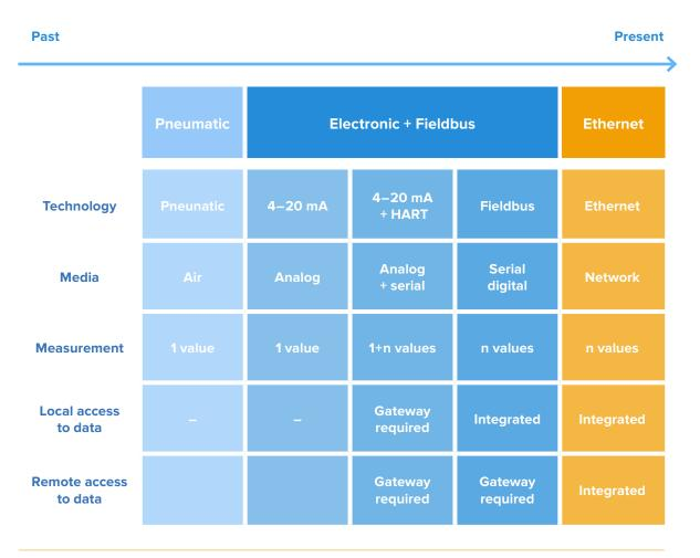
Figure 1: Technologies for the field of process automation
