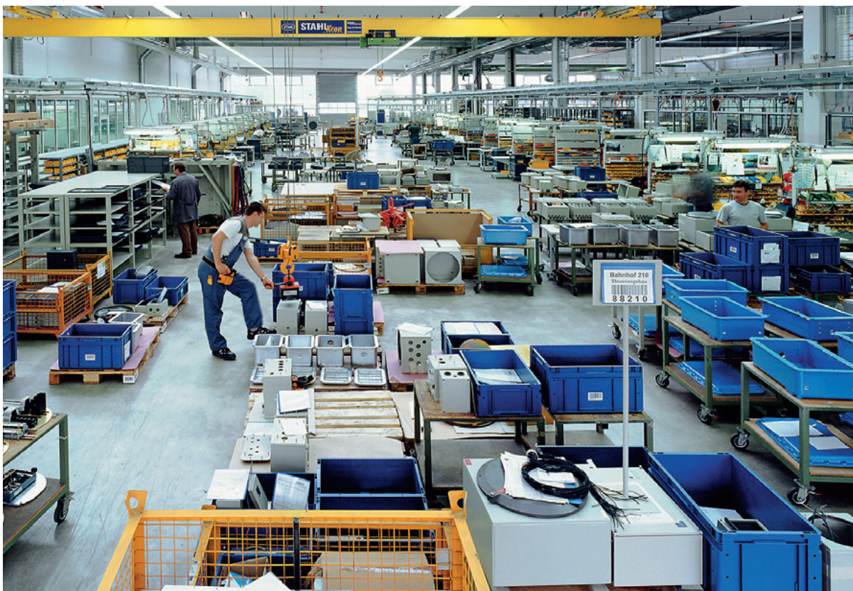
Flexible production line for control units at the Waldenburg facility. Thick-walled “Ex d” enclosures can be seen in the back right of the picture.
